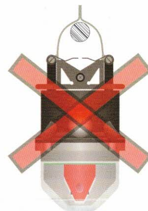
figure 4 - wrong cable position
