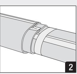
Install subsequent sections of mat, tightly butted up to preceding section, but still maintaining the overlap onto the cut edge a minimum of 50mm. Install additional layers, as required per system specifications, making sure to stagger joints a minimum of 50mm. Close all cut edges with 3M<sup>™</sup> Aluminum Foil Tape. E-Mat may be temporarily retained with 19mm wide filament tape.
