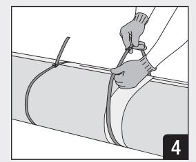
Tightly clamp minimum 13mm wide steel retention bands around E-Mat. Bands to be positioned 25mm from each joint and at the center of each width of E-Mat.
