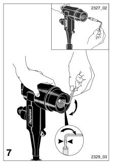
Insert the connection pin into the elbow and fasten it with the allen key. Apply enough torque until the allen key is deformed.
