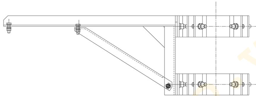
*27 kV/38 kV Mounting bracket assembly
