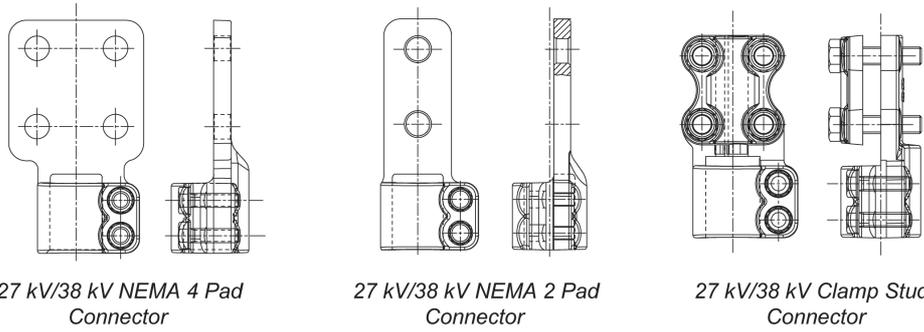
Either one of the above three connectors are required in 6 quantity or recloser.
